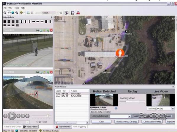
When the PTZ camera arrives at the target, the PureActiv video analytics is invoked to further assess the target. PureActiv video analytics can classify the target as human, vehicle or other and command the PTZ camera to automatically follow the target. When the Intrepid sensor and video analytics both report a positive detection, the probability of detection is much greater than a single sensor and the false alarm rate is also dramatically reduced.
