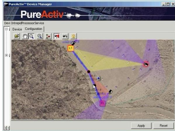
The same configuration process is used to define the physical locations of in-ground Microtrack and Volumetric microwave sensors within the PureActiv georeferencing map.
