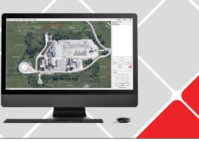
INTREPID<sup>™</sup> Graphic Alarm Manager (GAM) is a dedicated, Windows-based system controller with graphic mapping capabilities designed to provide GUI-based alarm monitoring and control of INTREPID<sup>™</sup> Series II and POE-S intrusion detection systems, contact closure auxiliary security devices and CCTV equipment via relays or output commands.
